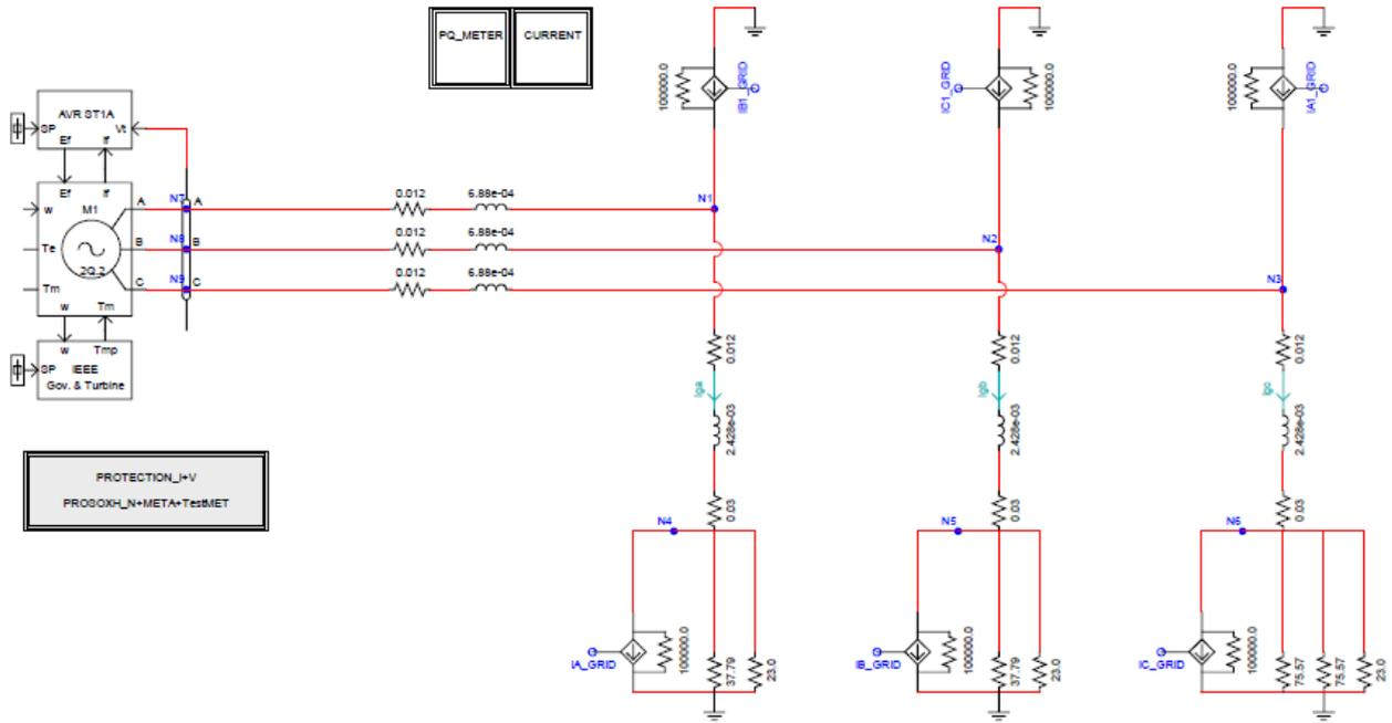
Figure 5. Simulated system in RSCAD/RTDS software environment.
