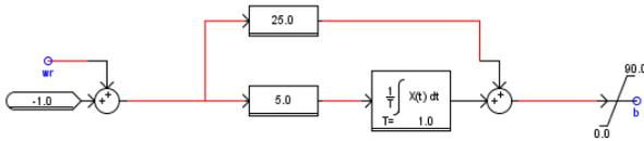
Figure 1. Pitch controller model in RSCAD/RTDS
