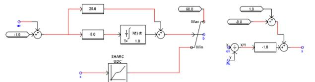
Figure 4. Pitch controller in pitch deloading mode.
