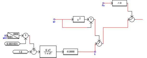
Figure 2. Inertia response input to the original model.
