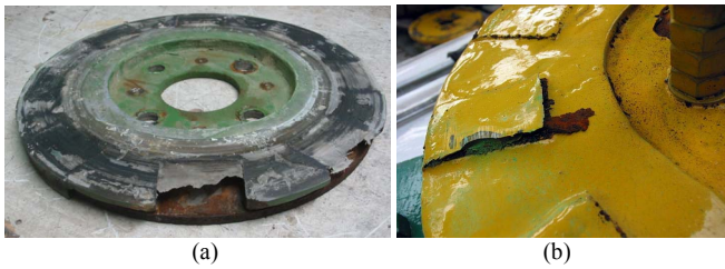
Fig. 1. Two cases of corrosion in locally manufactured SWTs (a) corrosion of the back iron disk, (b) corrosion of a NFeB magnet
