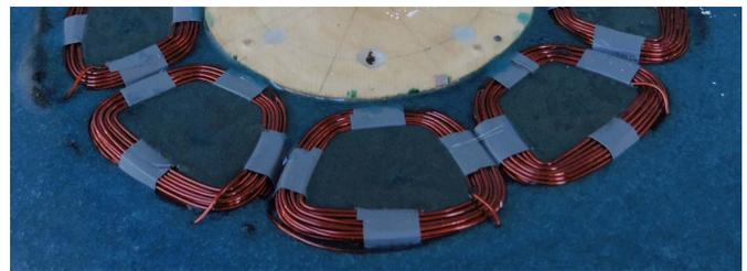
Fig. 3. The soft magnetic composite material mixed with vinyl ester resin and poured into the stator's concentrated windings.
