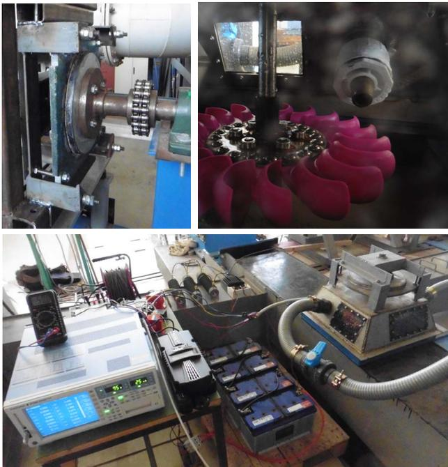
Fig. 8. The LMPHP tested in the hydraulics laboratory of the NTUA, a double-rotor single-stator AFPMG on the DC motor test bench and a locally manufactured 3D printed Turgo turbine.
