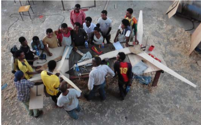
Fig. 8. Manufacturing a 3.6m LMSWT with students from the university of Semara in the Afar region of Ethiopia
